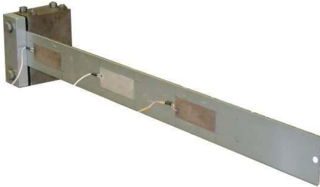
Fig. 1. Picture of the cantilever beam.
