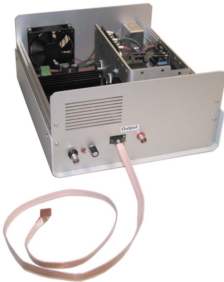
FIG. 3. (Color online) Amplifier enclosure with connected cable and 100 nF capacitive load.
