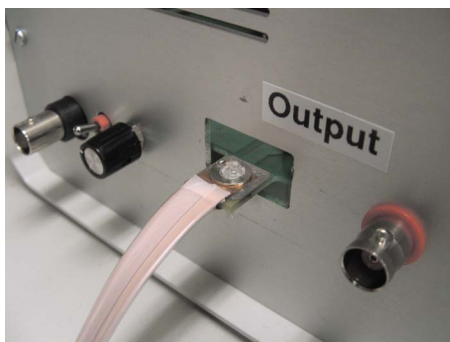
FIG. 7. (Color online) Close-up of low-inductance connection between amplifier circuit board and cable.
