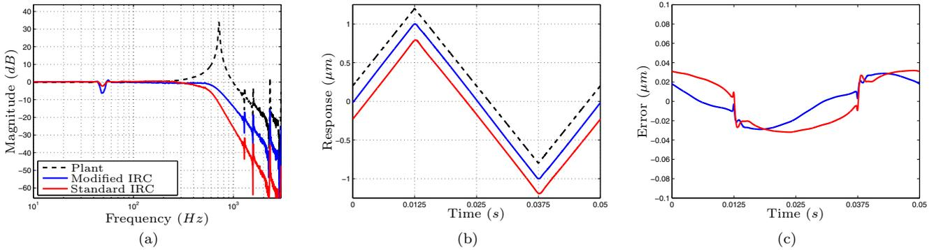
Fig. 3. (a) Bode magnitude plot for the plant, standard, and modified IRC schemes. (b) Simulated response of each of the IRC schemes to an input of a 20 Hz triangle wave of amplitude  $\pm 1 \mu m$ , offset by  $0.2 \mu m$  for clarity, and time-shifted to compensate for phase differences. (c) Error signals for both the standard and modified IRC schemes.
