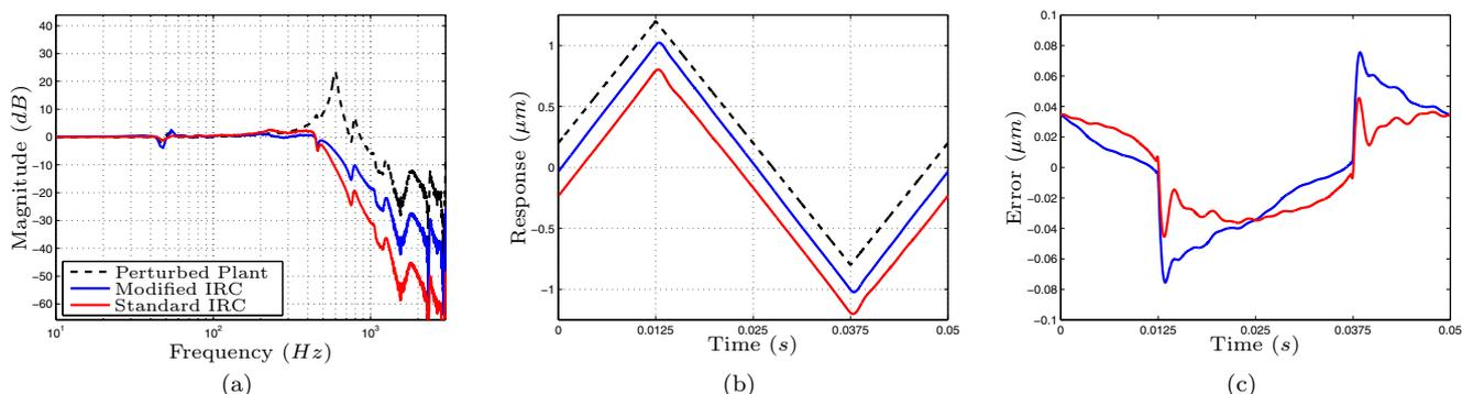
Fig. 4. (a) Bode magnitude plot for the perturbed plant, standard, and modified IRC schemes. (b) Simulated response of each of the IRC schemes to an input of a 20 Hz triangle wave of amplitude  $\pm 1 \mu\text{m}$ , offset by  $0.2 \mu\text{m}$  for clarity, and time-shifted to compensate for phase differences. (c) Error signals for both the standard and modified IRC schemes.
