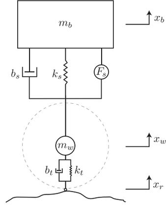
Fig. 1: Idealised quarter-car suspension system.
