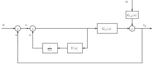
Fig. 2.3. The feedback structure associated with the shunt damping problem in Figure 2.2
