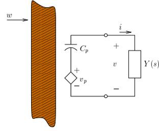
Fig. 2.2. Electrical equivalent of the system in Figure 2.1
