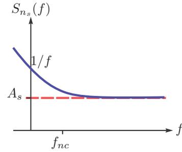
Fig. 2. Power spectral density of a baseband sensor (solid line) and a modulated sensor (dashed line).  $A_s$  is the noise density and  $f_{nc}$  is the  $1/f$  noise corner frequency.
