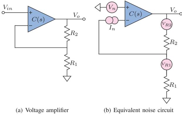
Fig. 3. The simplified schematic of a voltage amplifier and its equivalent noise circuit. The noise sources  $V_n$  and  $I_n$  represent the equivalent input voltage noise and current noise of the amplifier.  $V_{R1}$  and  $V_{R2}$  are the thermal noise of the feedback resistors.
