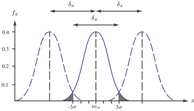
Fig. 1. The random motion of a two-dimensional nanopositioner. The random motion in the  $x$  and  $y$ -axis is bounded by  $\delta_x$  and  $\delta_y$ . In the  $x$ -axis, the standard deviation and mean are  $\sigma_x$  and  $m_x$  respectively. The shaded areas represent the probability of the position being outside the range specified by  $\delta_x$ .
