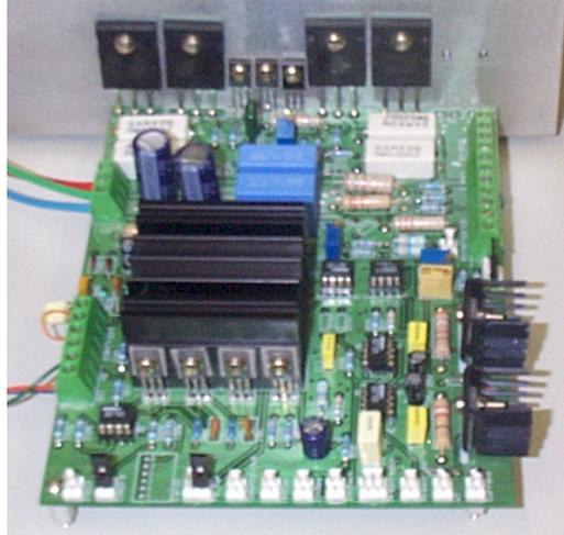
**Figure 9.** Photograph of a prototype current / charge amplifier.
