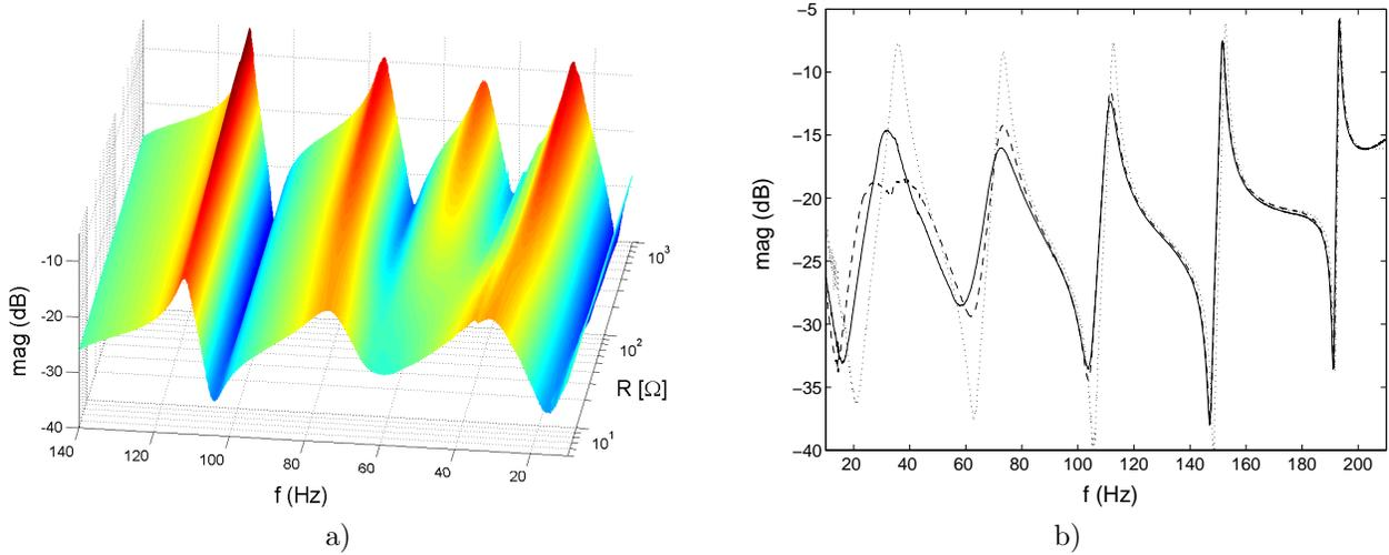
**Figure 8.** Measured magnitude of the transfer-function  $G_{p1\nu1}$ . a) Passive  $R$  shunt b) Passive  $R//C$  shunt. (...) duct without speaker, (—) duct with open speaker, (- -) duct with  $C//R$  shunt tuned to the 1<sup>st</sup> mode.
