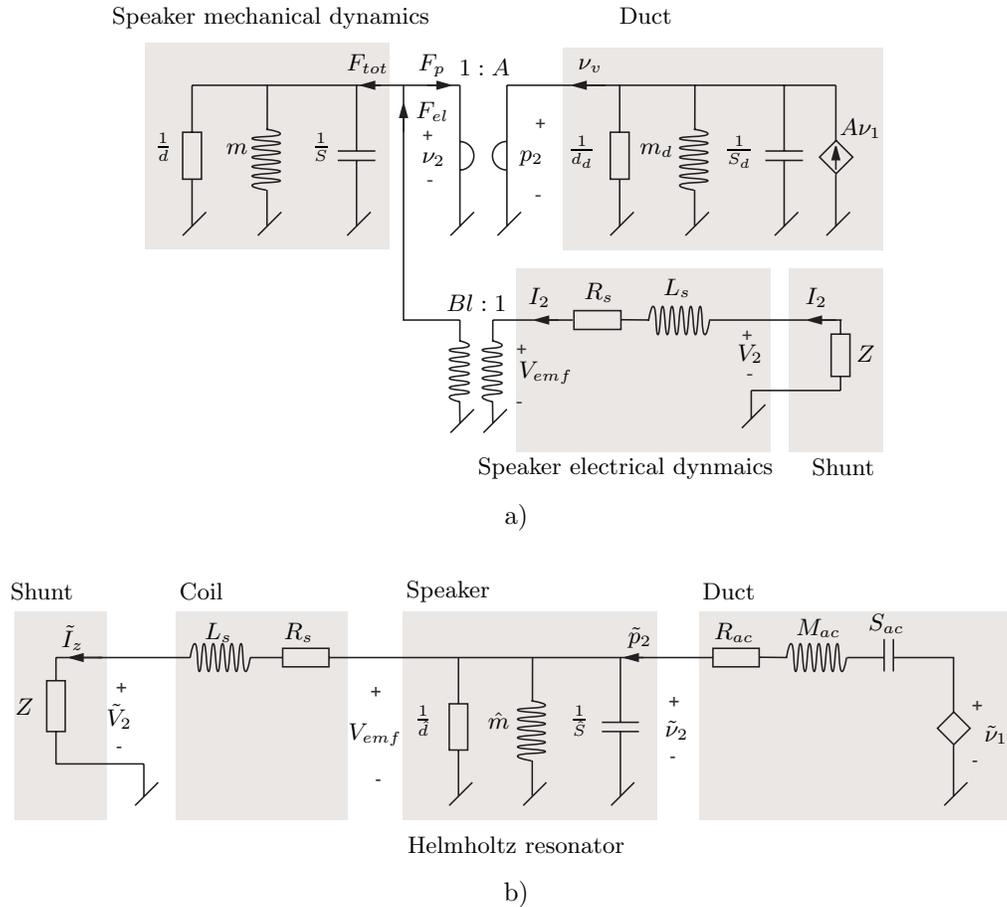
**Figure 7.** a) Electrical equivalent model of the composite speaker-enclosure system. b) simplified electrical equivalent.
