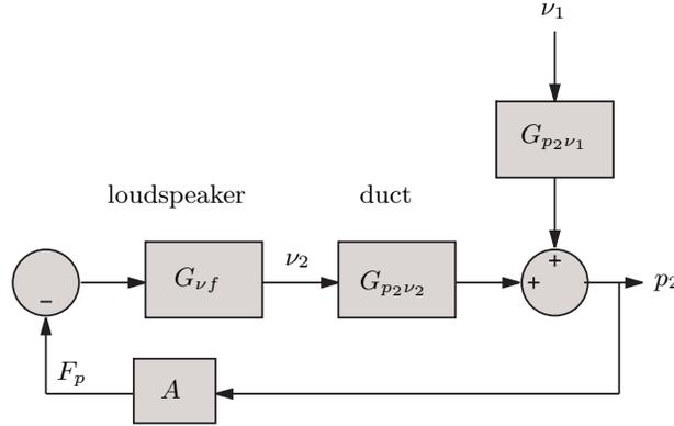
**Figure 4.** Block diagram of the composite acoustic and passive loudspeaker dynamics.
