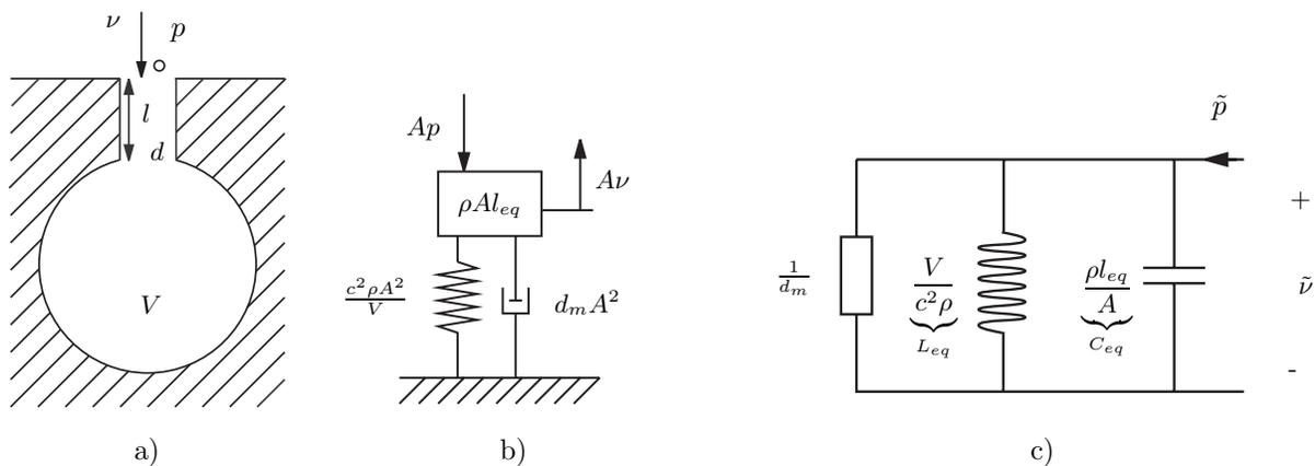
Figure 6. a) Sketch of the Helmholtz resonator, b) Equivalent mechanical model and c) equivalent electrical model.
