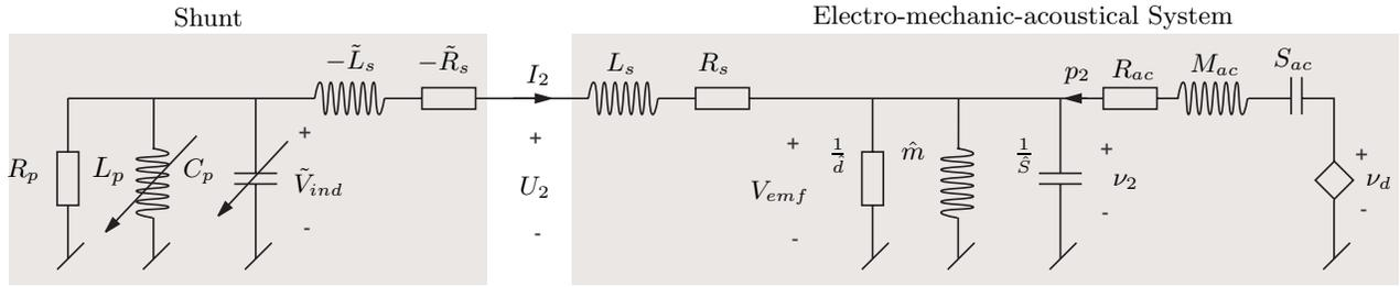
**Figure 9.** Shunt with negative  $R_s - L_s$  and parallel  $R//L//C$  network. All virtual Helmholtz parameters can be varied.
