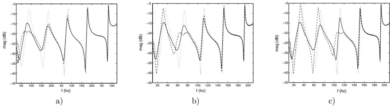
**Figure 10.** Negative  $R_s - L_s$  with  $R//L//C$  shunt. The shunt circuit is tuned to a) 1<sup>st</sup> mode, b) 2<sup>nd</sup> mode and c) 3<sup>rd</sup> mode. (...) duct without speaker, (—) duct with open speaker, (- -) duct with shunt.
