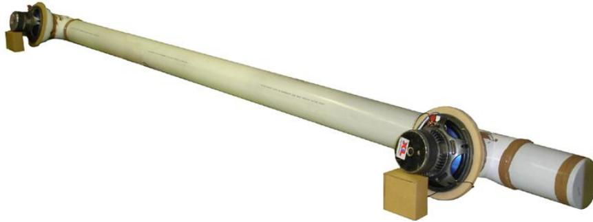
**Figure 1.** Experimental duct with two transversely mounted loudspeakers
