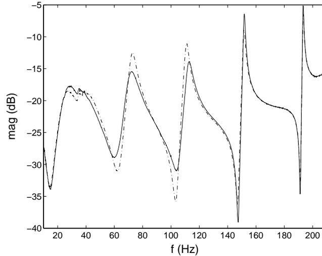
**Figure 11.** Measured magnitude of the transfer-function  $G_{p_1 \nu_1}$  using negative  $\tilde{R}_s - \tilde{L}_s$  with  $R_p // L_p // C_p$  and serial  $L$  shunt to improve damping of higher modes. ( - - ) negative  $R-L$  with  $R // L // C$  shunt, ( — ) improved shunt with additional series inductor.
