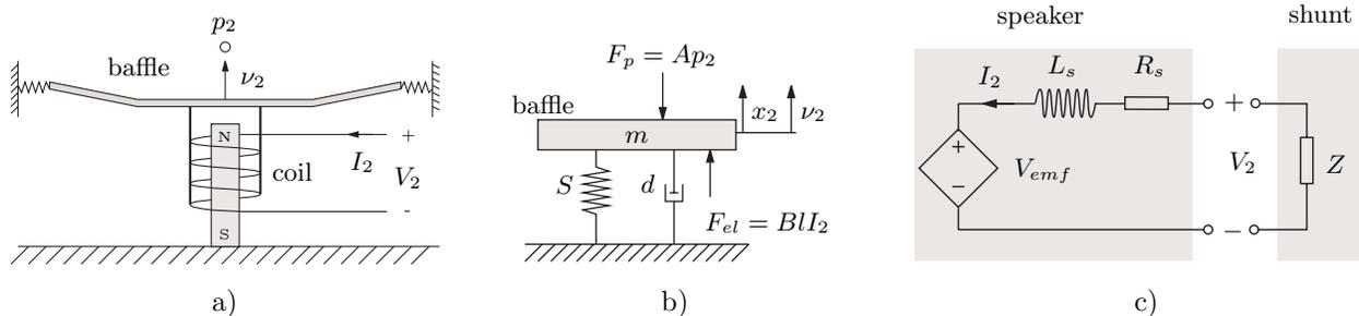
**Figure 3.** a) Sketch of the speaker, b) Mechanical equivalent diagram c) Electrical equivalent diagram
