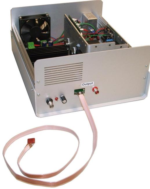
**Figure 3.** Amplifier enclosure with connected cable and 100 nF capacitive load
