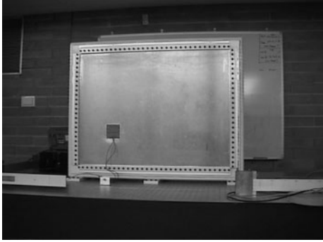
Figure 8. Piezoelectric laminated plate bounded structure.
