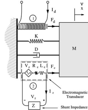
Fig. 1. Electromagnetic shunted mass spring damper system.
