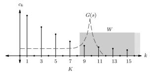
Fig. 6. Fourier components of a triangular scanning signal plotted against harmonic number k. The optimal signal is unrestricted in spectral content between dc and the Kth harmonic. All harmonics greater than K are penalized to avoid excitation of the system G.
