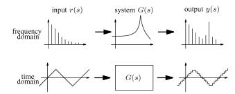
Fig. 1. Triangular scanning signal distorted by a typical mechanical system.
