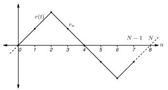
Fig. 3. Periodic signal r(t) and its samples  $r_n$ .
