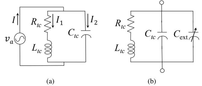
Fig. 3: (a) Equivalent circuit of a transmitter (b) Circuit diagram to estimate  $C_{tc}$  by applying the resonance method.
