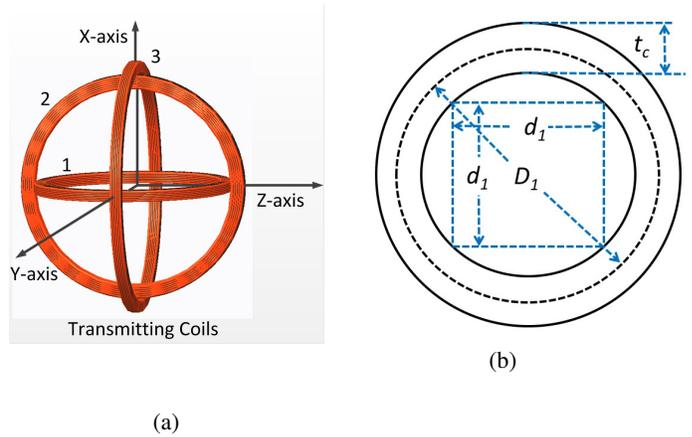
Fig. 8: (a) Concentric, orthogonal transmitting coils, and (b) the cross-sectional view of the innermost coil.
