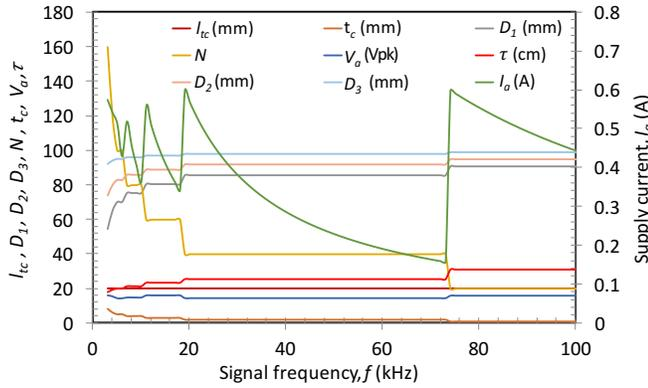
Fig. 9: Optimized transmitting coil dimensions when the length of the transmitting coils is fixed at 20 mm. The values at 74.1 kHz are considered to be optimal since the transmitting coil is single layer and the sensing range  $\tau$  is maximum at that frequency.
