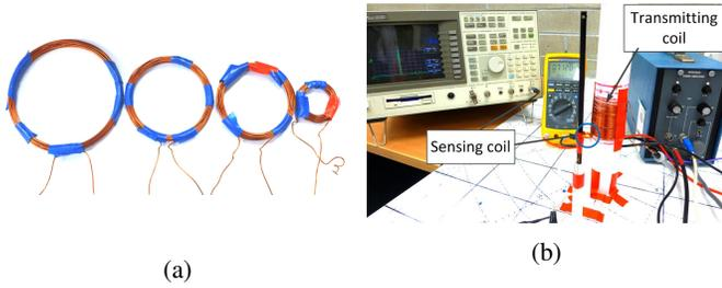
Fig. 5: (a) Various transmitting coils used to test the impact of radius on induced voltage. (b) Experimental setup for testing the impact of signal frequency, current, voltage, and the number of turns in the transmitting coil on induced voltage.
