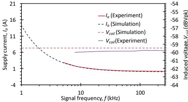
Fig. 6: Simulation and experimental results that illustrate the relationship between the induced voltage in the sensing coil and the signal frequency and current.
