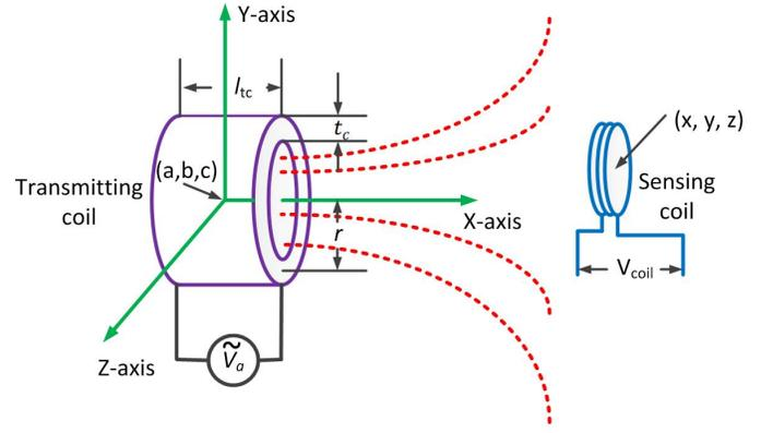
Fig. 2: Electromagnetic induction in the sensing coil due to a magnetic dipole which is parallel to the X-axis
