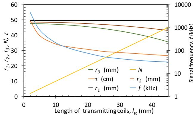
Fig. 10: Optimized transmitting coil dimensions as a function of length, and the achievable sensing ranges  $\tau$  at different signal frequencies.  $V = 15$  Vpk,  $I = 0.6$  A,  $t_c = 1$  mm,  $l_{tc} = 1 \sim 45$  mm. The radius of the transmitting coils are  $r_1$ ,  $r_2$  and  $r_3$ .
