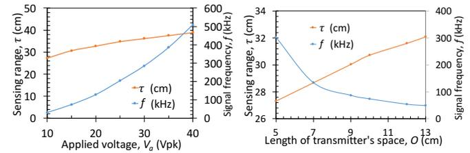
(a)  $P = 9$  W,  $V_a = 10 \sim 40$  Vpk, (b)  $P = 9$  W,  $O = 5 \sim 13$  cm,  $l_{tc} = 20$  mm,  $O = 10$  cm  $l_{tc} = 20$  mm,  $V_a = 15$  Vpk
