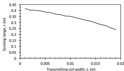
Fig. 12: The relationship between the transmitting coil width and system range.
