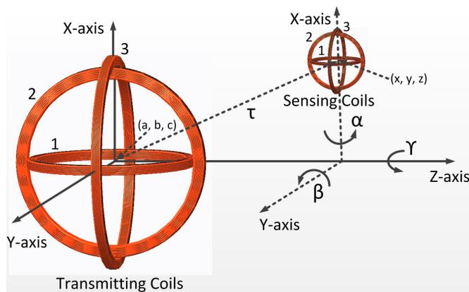
Fig. 1: A 6-DOF electromagnetic (EM) tracking system
