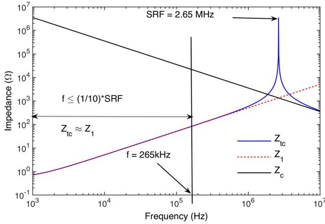
Fig. 4: Impedance characteristics of a transmitting versus frequency.  $L_{tc} = 80 \mu\text{H}$ ,  $C_{tc} = 45 \text{ pF}$ ,  $\text{SRF} = 2.65 \text{ MHz}$
