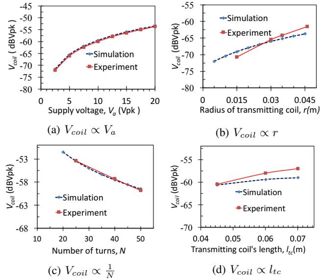
Fig. 7: Variation of induced voltage in the sensing coil due to the variation of (a) applied voltage, (b) the radius of the transmitting coil, (c) the number of turns in the transmitting coil, and (d) the length of the transmitting coil.
