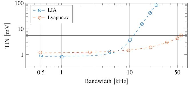
Fig. 7. Measured TIN of amplitude estimate from LIA and Lyapunov estimator, with curve fit, as a function of tracking bandwidth.
