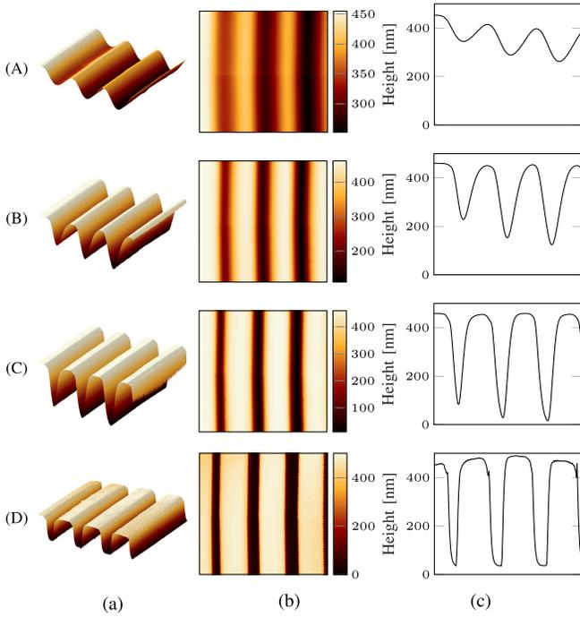
Fig. 8. AFM scanning results. (A) LIA with  $f_c = 100$  Hz, (B) LIA with  $f_c = 200$  Hz, (C) LIA with  $f_c = 400$  Hz, and (D) Lyapunov estimator with  $\gamma = 60 \times 10^3$ , providing a tracking bandwidth of  $\sim 1.6$  kHz. (a) 3-D Image. (b) 2-D Image. (c) Cross section.
