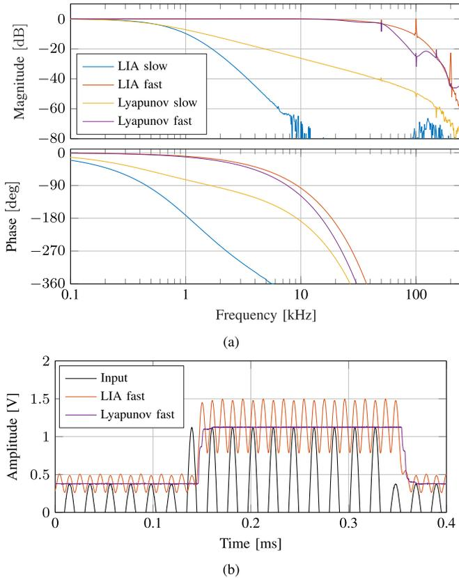
Fig. 5. Amplitude tracking experiment using the LIA and Lyapunov estimator with a carrier frequency of 50 kHz. (a) Frequency response at different bandwidth settings. (b) Time-domain tracking of a square-modulated sine wave.
