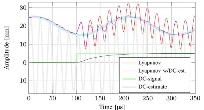
Fig. 4. Lyapunov estimator simulated with a step in dc-offset at the input signal, with carrier frequency  $f_0 = 50$  kHz, gain  $\gamma = 9 f_0$ , and dc-gain  $\gamma_{dc} = 20$  k for the augmented Lyapunov estimator with dc-estimation.
