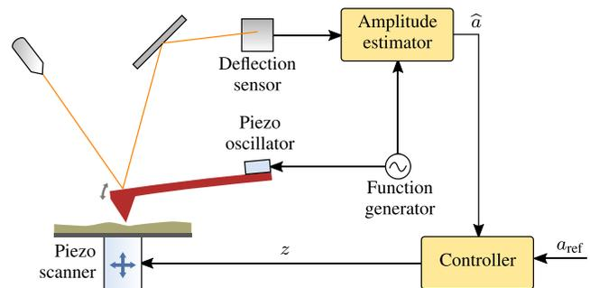
Fig. 1. Amplitude modulated operating mode in AFM.
