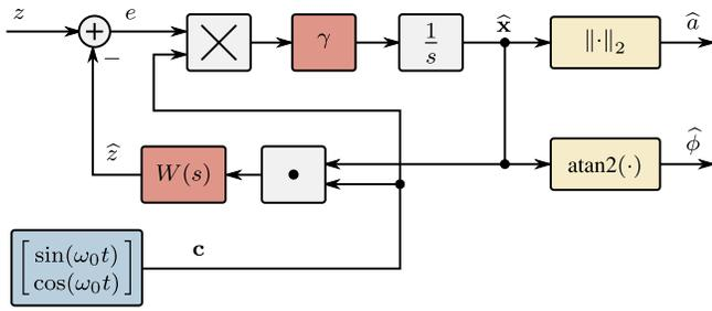
Fig. 2. Block diagram of the estimator. The blocks “ $\cdot$ ” and “ $\times$ ” represent vector dot product and matrix multiplication, respectively.
