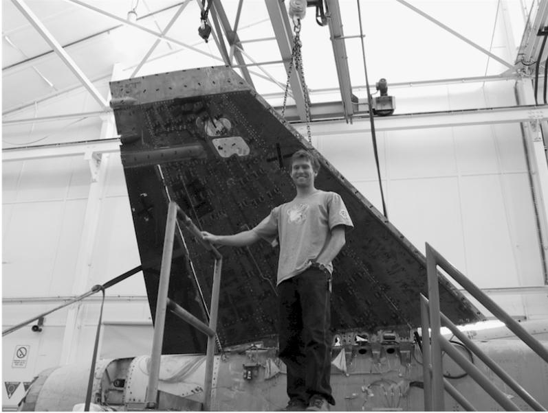
**Figure 1.7:** A piezoelectric laminate FA-18 vertical stabilizer. The author is in the foreground (Courtesy of T. Ryall, DSTO, Fishermans Bend).
