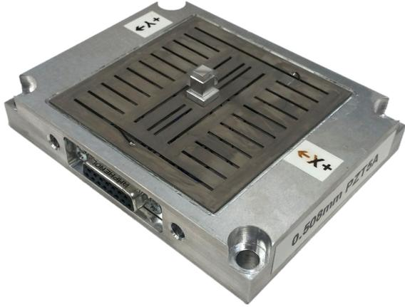
(a) The machined piezoelectric sheet forming the nanopositioner.
