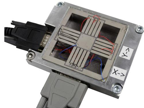
Fig. 1. Monolithic bi-morph nanopositioner mounted on a base.
