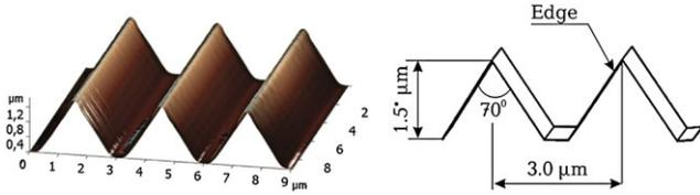
Fig. 12. An NT-MDT TGG1 calibration grating. The grating has a triangular step profile with a height of  $1.5 \mu\text{m}$  and a period of  $3.0 \mu\text{m}$ . [Color figure can be viewed at wileyonlinelibrary.com]
