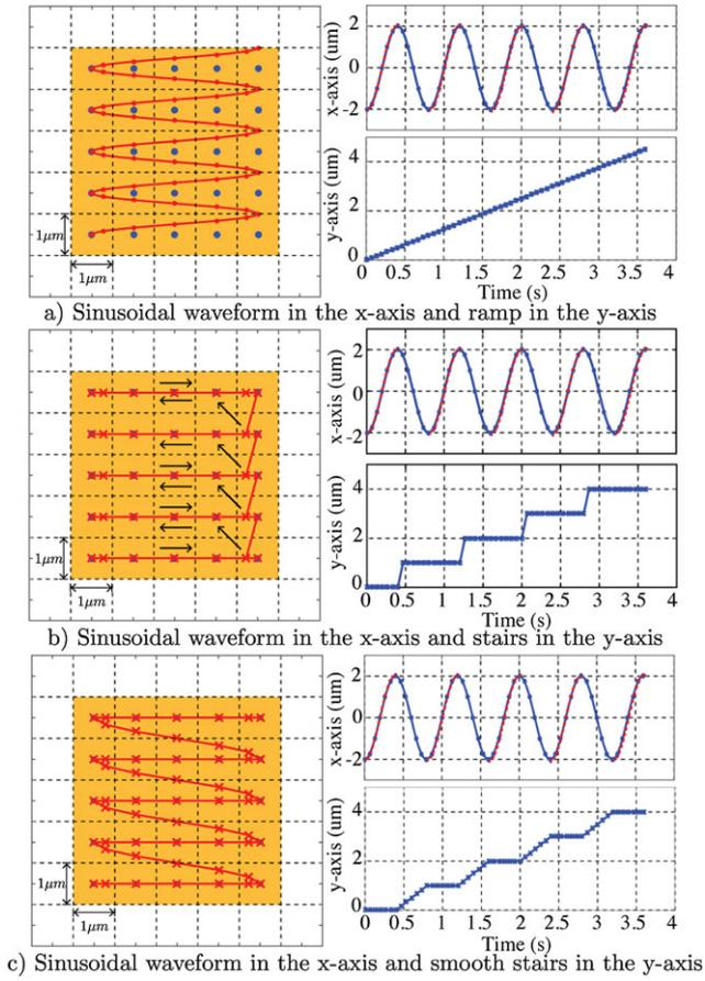
Fig. 4. A comparison of different sinusoidal raster scan methods in the y-axis. [Color figure can be viewed at wileyonlinelibrary.com]
