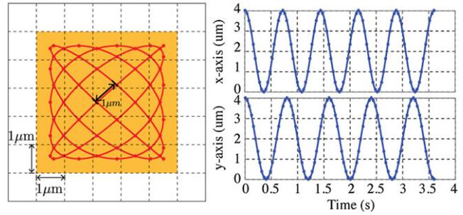
Fig. 6. Lissajous scan of a  $5 \mu\text{m}$  image. [Color figure can be viewed at wileyonlinelibrary.com]
