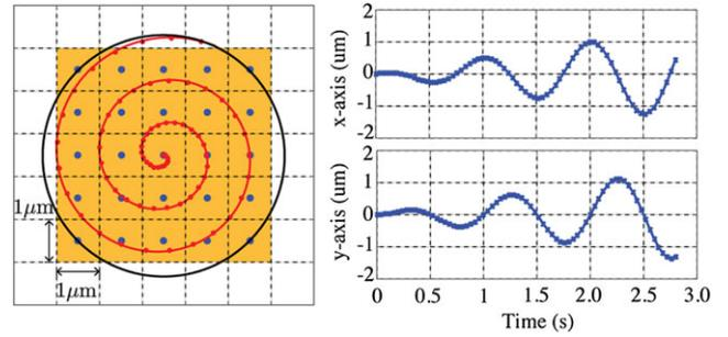
Fig. 5. Spiral scan of a  $5 \mu\text{m}$  image with constant angular velocity. [Color figure can be viewed at wileyonlinelibrary.com]
