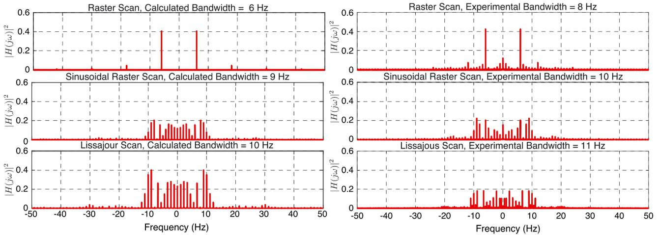
(a) Case 1: The frequency spectrum in the topographic signal for each scanning methods with an imaging time of 256 s. Simulation results (left), experimental results (right).
