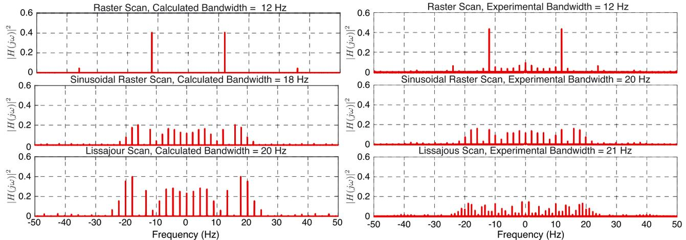
(b) Case 2: The frequency spectrum in the topographic signal for different scanning methods with an imaging time of 128 s. Simulation results (left), experimental results (right).
