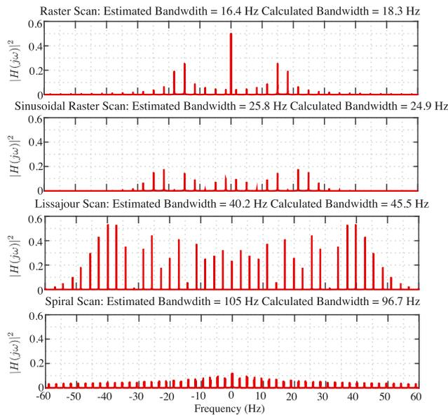
Fig. 9. The frequency spectrum of the topography signal  $h(t)$ . [Color figure can be viewed at wileyonlinelibrary.com]
