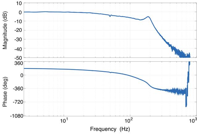
Fig. 11. Measured closed-loop frequency response of the vertical stage in the Nanosurf positioner. The measurement was performed while maintaining constant contact force between the probe tip and sample grating. [Color figure can be viewed at wileyonlinelibrary.com]
