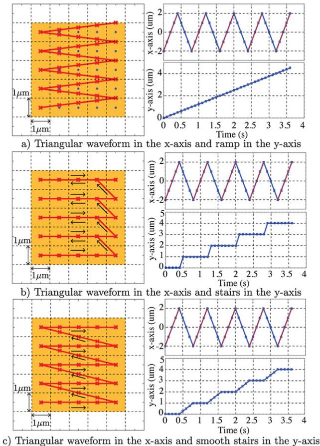
Fig. 2. A comparison of different raster scan methods in the y-axis. [Color figure can be viewed at wileyonlinelibrary.com]
