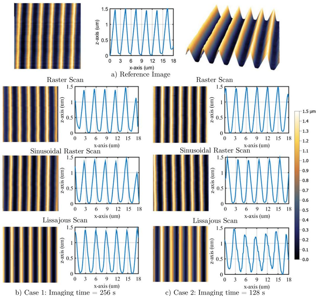
Fig. 13. (a) A reference image of the TGG1 calibration grating. (b) The profiles and topographies for raster, sinusoidal raster and Lissajous scans for a fixed imaging time of 256 s. (c) The profiles and topographies for raster, sinusoidal raster and Lissajous scans for a fixed imaging time of 128 s. [Color figure can be viewed at wileyonlinelibrary.com]
