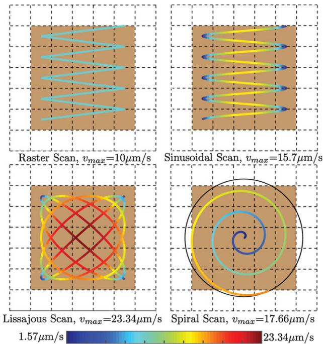
Fig. 7. A comparison of the velocity for a  $5 \times 5\mu\text{m}$  scan with  $1\mu\text{m}$  resolution and an imaging time of 3.6 s. [Color figure can be viewed at wileyonlinelibrary.com]
