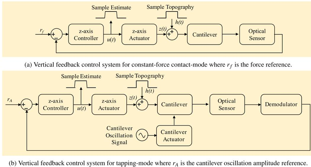
(a) Vertical feedback control system for constant-force contact-mode where  $r_f$  is the force reference.
